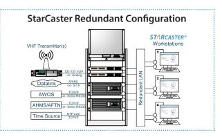
Intended for airports of all sizes, **STARCASTER**<sup>®</sup> is scalable from a single workstation configuration to a fully redundant system to ensure high availability.
